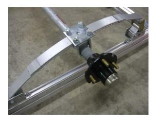
Install the U-bolts as shown. Make sure the stud on the spring aligns with the hole in the middle of the tie plate. Do not tighten the nuts yet.
