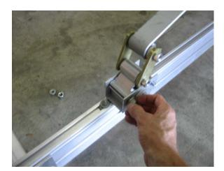
Install the spring assembly with the shackle holder to the rear of the trailer and the nuts to the inside.
