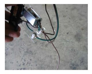
Strip the wires and install the 3 brown wires and 1 green wire onto the color matching wire terminals on the bulb assembly.
