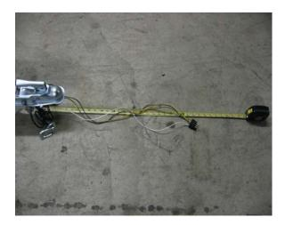
Pull the wires from the back of trailer until approximately 30" of wire is protruding at the front.
