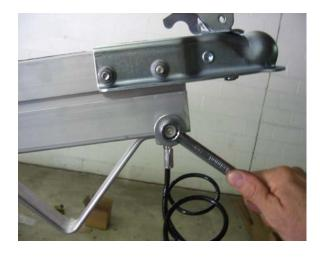
Rotate the safety cables so they point straight down and tighten.
