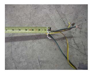
Attach the end of the harness to the tape measure using the tie wrap from the wire harness.
