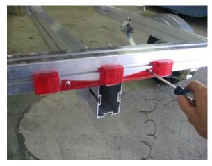
Install the three light bar using the screws located on the rear cross member.
