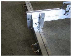
Attach the side rail to the brackets making sure the bracket is flush with the end of the side rail.
