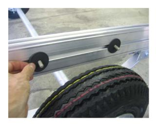
Install 2 rubber washers onto the T-bolts.
