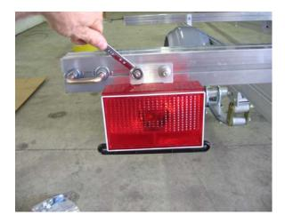
Tighten the tail light in this position. Repeat for the other side.
