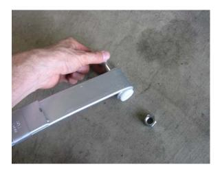
Remove the bolt from the front spring eye.
