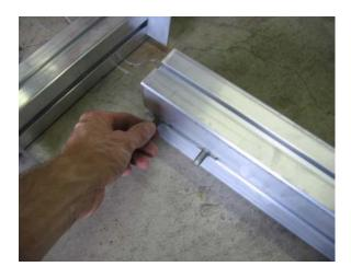
Slide the 4 T-bolts that were removed from the brackets into the tongue section from the rear (2 per side).
