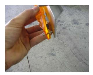
Install the running light on the bracket making sure the screw goes through the ring terminal on the white wire.
