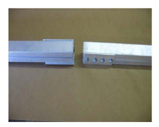
Lay the two tongue section adjacent to each other as shown. The splice plates should be positioned on the sides and bottom.
