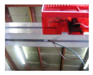
Route the green/brown wire together with the wire from the three light bar in the slot at the bottom of the rear cross member to the right tail light using adhesive clamps as shown.
