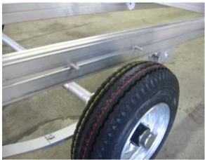
Install 2 T-bolts in the side rail and slide them forward until they are located over the tire.
