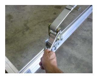
Tighten the shackle link nuts until there is a slight restriction in the movement of the shackle link.
