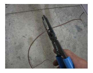
Cut the wire and strip 1/4" of insulation from the end.
