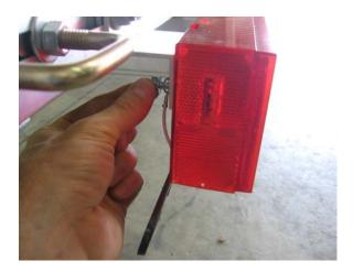
Bring the white wire around to the rear of the tail light and install it on the bolt. Do not over tighten the nuts.
