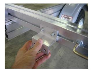
Install the brackets onto the T-bolts located in the rear cross member. Do not tighten.
