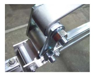
On the rear shackle, do not over tighten as this will not allow the suspension to move properly.
