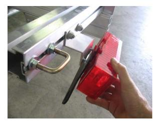
Install the left tail light with the license plate holder between the light and the bracket.
