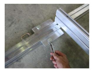
Remove the T-bolts from the side rail attaching angles on the cross members.
