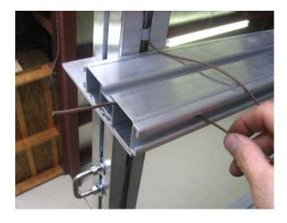
Route the remaining brown wire that will power the running light back along the rear cross member, through the adhesive clamps, and into the hole in the bottom slot of the side rail exiting out of the rear as shown.
