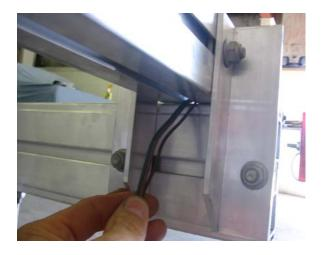
Route the wires between the rear cross member and the side rail.
