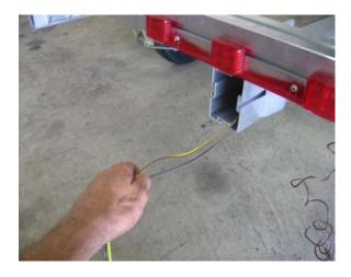
Retract the tape until the harness comes out of the back of the tongue.
