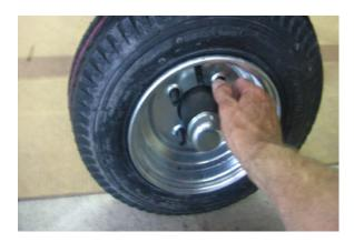
Install the wheels with the valve stems facing out. Install the lug nuts with the tapered side facing the wheel. Tighten to 80 foot pounds in a crossing pattern. Re-tighten after 25 miles. Recommended tire pressure is 25psi.
