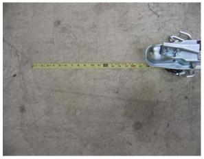
From the back of the trailer extend a tape measure through the tongue until it protrudes out of the front under the coupler.
