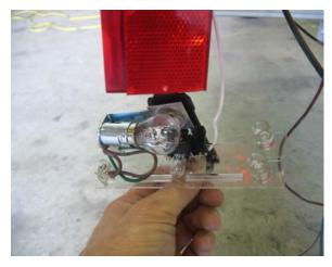
Remove the bulb assembly from the tail light by pulling the black tab toward the rear of the trailer and downward.
