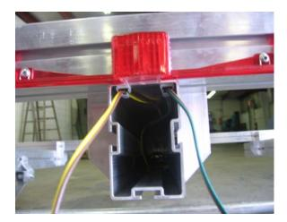
Install 2 clamps in the rear of the tongue as shown. Route the yellow wire through the left (driver's side) clamp, and the green wire through the right (passenger side) clamp.
