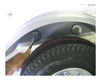
Install the steel washers and nuts. Center the fender over the tire and tighten the nuts. Repeat for the other side.
