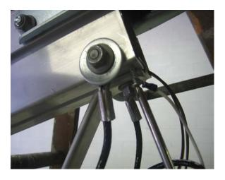
Crimp a ring terminal onto the white wire at the front of the trailer and install it into the pre-drilled hole located under the coupler.
