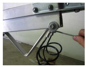
Install the skid into the slot in the bottom of the tongue.
