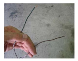
Take the excess green/brown wire that was cut off and separate the green wire from the brown wire. Discard the green wire. The single brown wire will be used to supply the running light.
