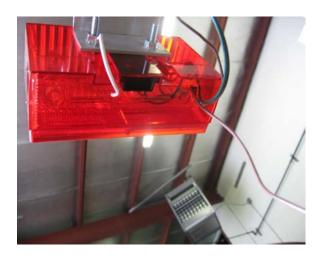
Re-install the bulb assembly into the tail light housing making sure to route the wires through the slot in the base of the bulb assembly.
