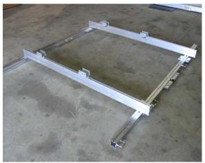
Place the side rails onto the cross members with the spring hangers toward the rear of the trailer.
