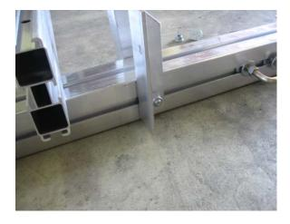
Rotate them upward making sure to align the brackets with the pencil marks on the cross members.
