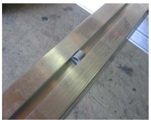
**Illustration: Adhesive clamp installed in slot.**
