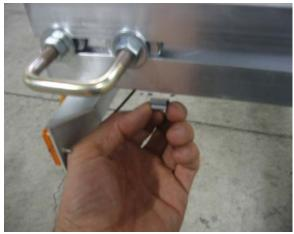
Install adhesive clamps to secure the wires in the slot on the bottom of the front cross member. Repeat the wiring procedure for the other side.
