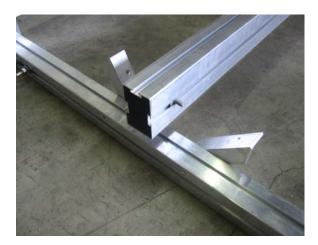
Lay the tongue onto the frame (remember the trailer is still upside down) making sure the rear of the tongue is flush with the back of the rear cross member.
