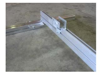
The spring hangers should be to the inside of the trailer.
