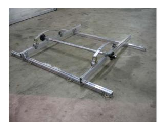
Lay the axle between the springs and the side rails with the axle's serial number plate toward the rear of the trailer.
