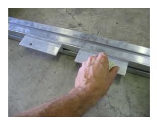
Remove 4 T-bolts from the tongue attaching brackets on the cross members..
