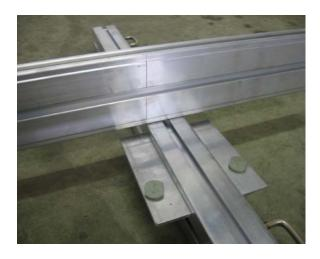
Align the rear edge of the front cross member with the pencil mark on the side rail. Repeat the procedure to attach the brackets to the side rail.
