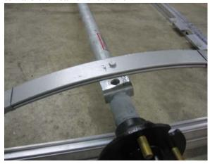
Raise the axle up and align the hole in the spring seat with the bolt in the spring.
