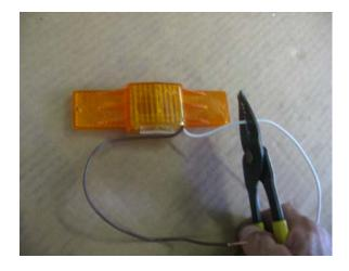
Cut approximately 8  $\frac{1}{2}$ " off of the white wires on both running lights.
